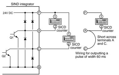
Figure 3-2 Connecting the SICD Counter
