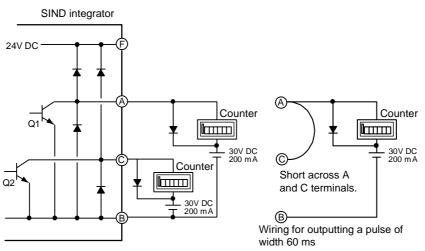
Figure 3-4 Connecting a Counter
