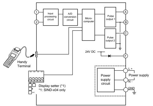
Figure 4-1 Hardware Function Block Diagram
