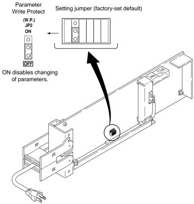
Figure 5-2 Parameter Write Protect Jumper
