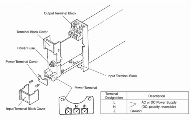
Figure 1 Names of Parts and Power Terminal
